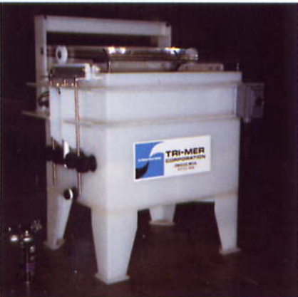
Custom tank with automated cover, spargers, heaters and controls.
