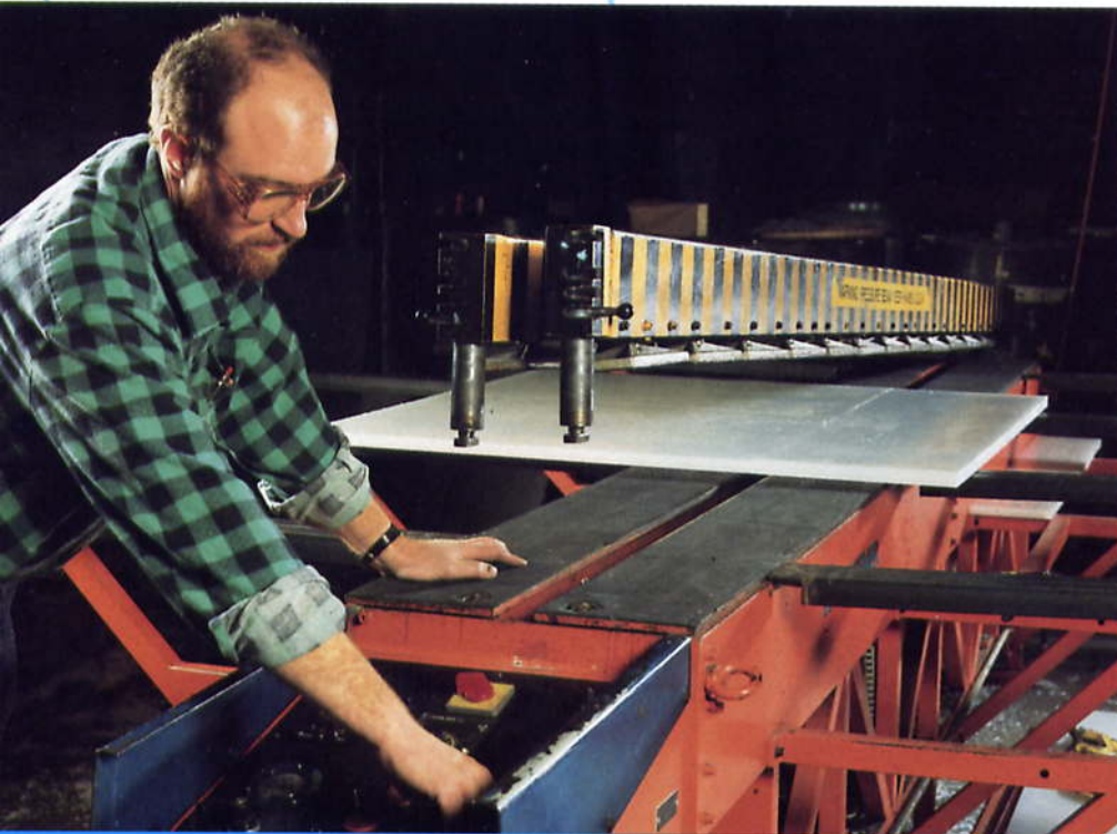
Automatic welding machine joining flat sheet polypropylene.
