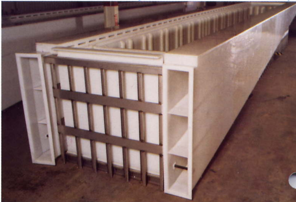
Large 48' long pickling tank with built-in exhaust hoods complete with stainless cradle shipped as an assembly.
