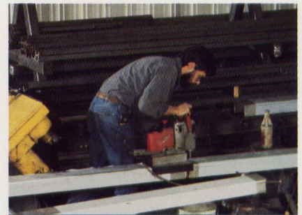
Fabricating stainless steel supports.
