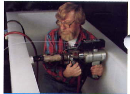
Technician with extrusion welder fabricating tank flange.
