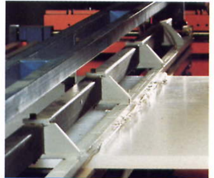
Automatic bending machine forming tank corner.
