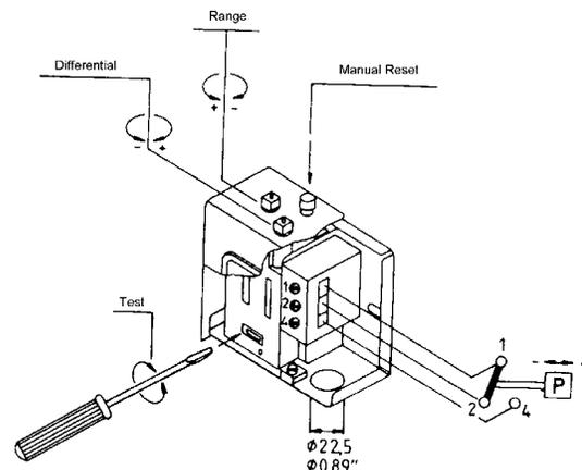
**NOTE:** The cut-in (start point) pressure is the cut-out (range adjusting setting) pressure minus the differential setting.
