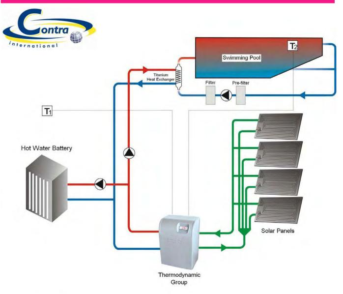
T1: Ambient Thermostat T2: Swimming Pool Thermostat
